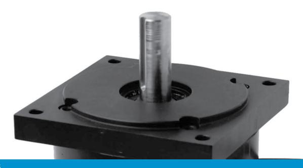
AMETEK offers power off, fail safe holding brakes to compliment its motor product line. When voltage is applied, the friction disc is released and the brake is free of torque. This power-off brake is best suited for parking brake applications used to hold a load in position, and is ideal for creating brake motor packages for small servo & stepper frame motors.
